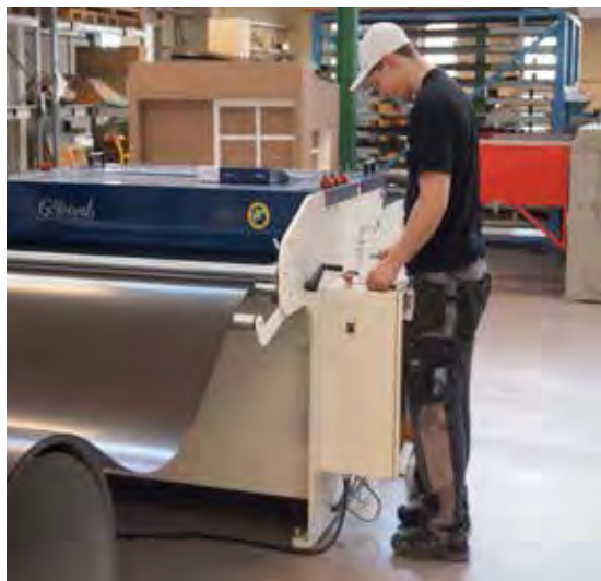
Leveling and cut-to size machine.
