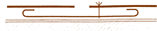
Joint - edge to edge with a sealing strip. This arrangement is used for preference when thick sheet metal is used.
